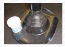
1 Cut the Fix-R EPDM PS Pipe Seal above the raised "rib" one size smaller than the pipe diameter. DO NOT CUT THROUGH THE RIB. Pull pipe seal over pipe until base flange is in contact with the Fix-R EPDM membrane.
