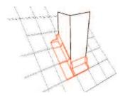
3. On side faces it is recommended that flashing is applied to each tile or slate separately.
