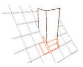
2. Flashing to all chimney faces should be joined by folding. Joints should have a minimum overlap of 100mm.
