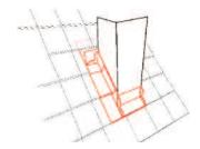
4. A roller is recommended to finish the application. It is also recommended to apply a roofing sealant to the connection at a chimney junction.
