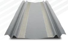
TIL-R Open Valley Troughs for Tile Roofs are made from GRP and provide secure drainage for inclined roof valleys. These troughs incorporate mortar bonding strips for tile bedding, and are designed with greater capacity suitable for both new build and refurbishment projects.
