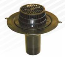
FIX-R Top Drain Is one of the best ways of connecting to a 110mm outlet drain. Its dimensions conform to UNI EN 1451-1 and it fits to bell and spigot jointed pipes without the use of adhesive. Top Drain is particularly suited for use in low sloping roofs, roof gardens, inverted roofs and box gutters. Fixing and fastening to the waterproofing material is by a threaded ring which allows for a fast, simple and watertight finish.
